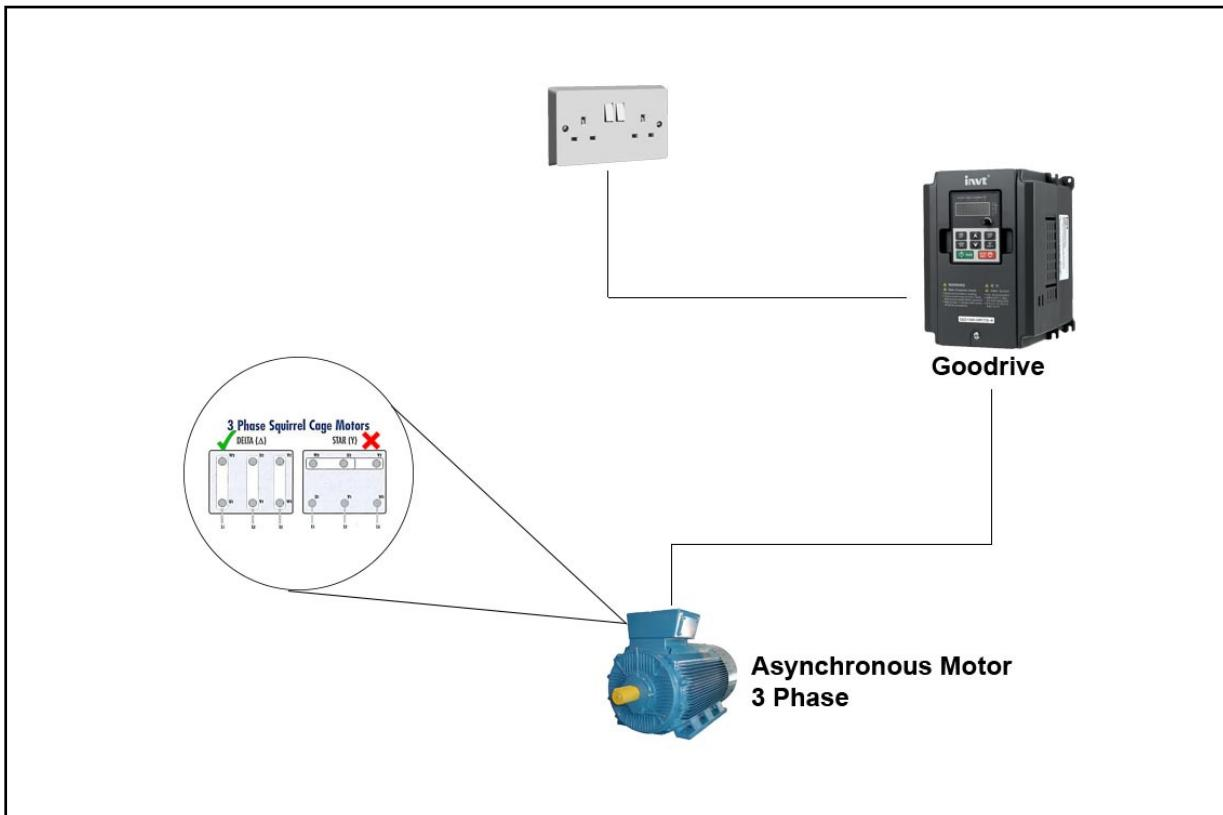
Our INVT Single Phase 220V Ac Inverters are capable of running 3 phase motors of 0,18kW or less and up to 4kW from a standard single phase wall supply.
