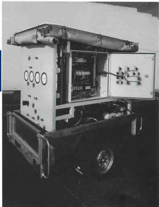
Typical Mobile SF 6 Gas Handling Carts
