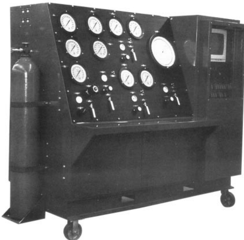
Natural gas driven natural gas amplifier system consumes no energy while providing direct fills to vehicle storage cylinders for natural gas powered vehicles.
