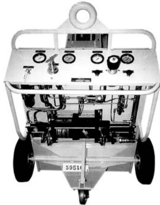
Two-wheel mobile N 2 charging unit
