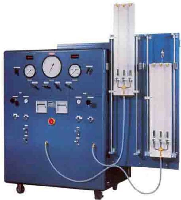
Gas cylinder stretch test rig complete with moveable burrettes
