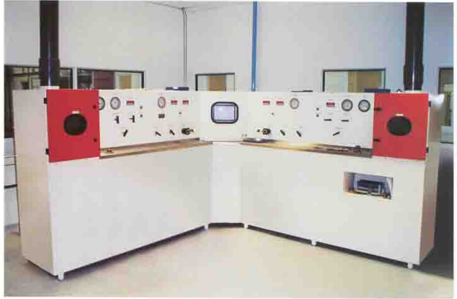
Relief valve 'pop and flow' test rig
