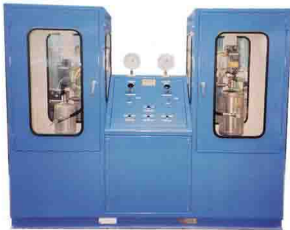
Two station air receiver water test rig
