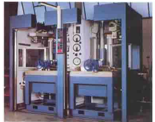
Two stations PLC controlled automatic valve test rig for gate valves up to 8" in diameter
