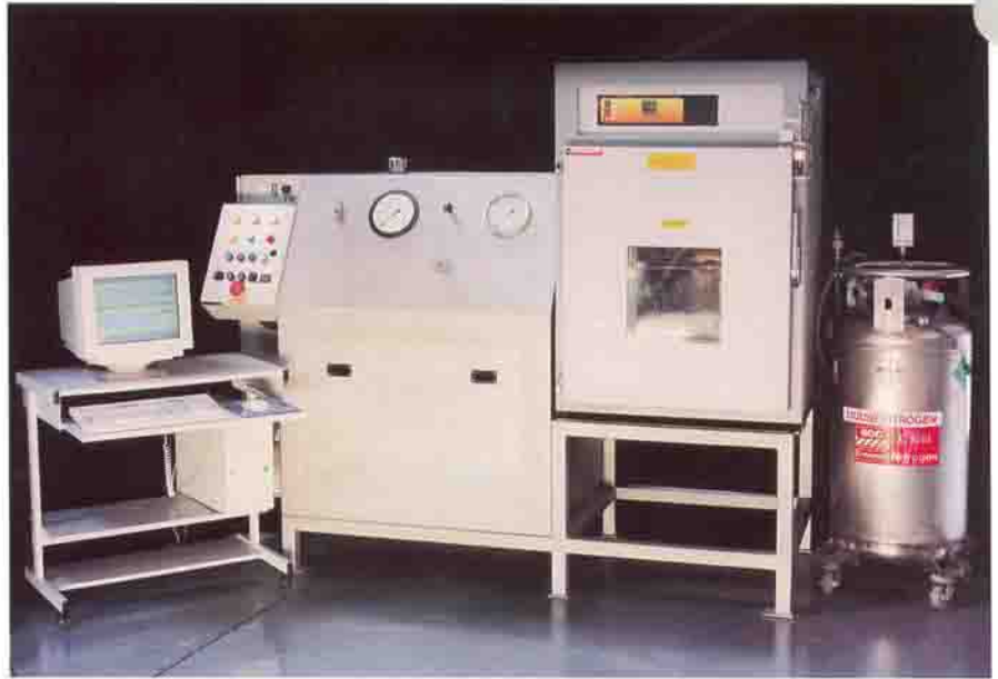
Temperature controlled burst and impulse test rig with environmental chamber. 240 bar, -40°C to +125°C
