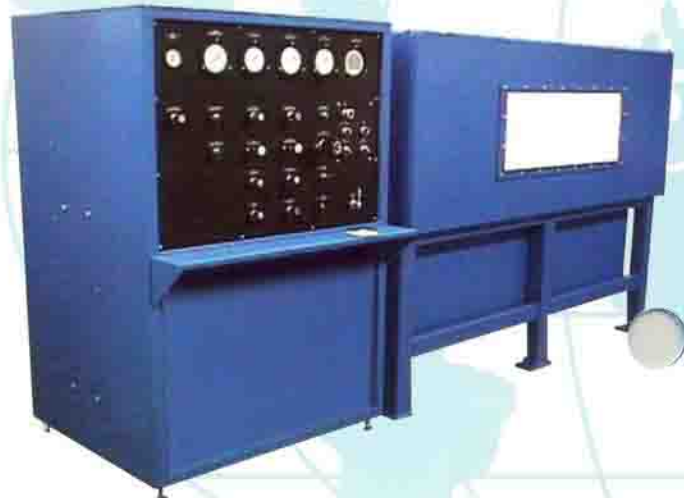
Multiple station hose test rig for hose assembly facilities up to 30,000 psi
