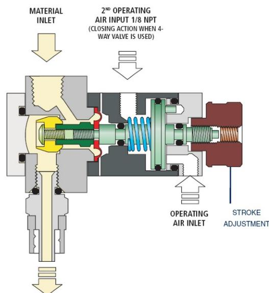
*Figure 4 – A cutaway schematic of a poppet dispensing valve, showing material flow path and operating air inlet. There is a stroke adjustment screw, and a second air inlet for an optional closing function.*
