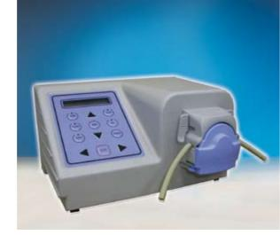
Programmable versions can dose single or repeat volumes with a user defined time interval between jobs. Accuracy with viscous products can be achieved using the calibration mode with a run-back option to prevent spillages. RS232 digital signal connection gives Windows based remote computer control of the pump providing the additional capability to store different pump settings.
